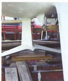
Right: The Starlight's optional winged keel. Note the well-protected prop shaft
